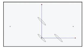
Figure 8: Layout and error ellipses for the free station geometry test observations and positions.
