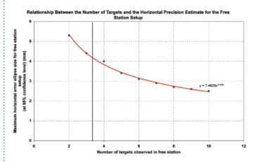
Figure 6: Relationship between the number of targets and the horizontal accuracy estimate for the free station setup
