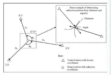
Figure 1: Free station procedure and processes
